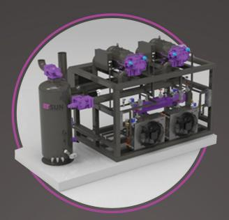
A parallel rack system is multiple compressor refrigeration units piped in parallel to yield smooth capacity control as compared to a single compressor unit.
